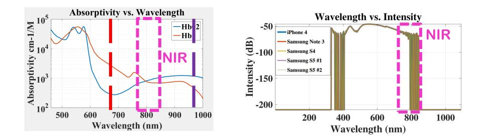
NIR has similar characteristics of hemoglobin absorption with the IR lights. is available in most of phone's flashlight and is not filtered by the phone's camera.
