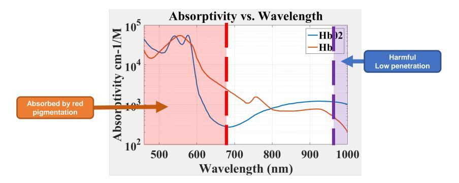
At Red= 660 nm and IR = 960 nm, the difference of light absorption by oxygenated hemoglobin and deoxygenated hemoglobin is largest.
